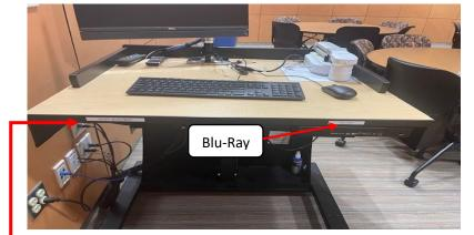
To adjust the height of the console, grasp the adjustment handle and squeeze towards you to release the mechanism. You can then raise or lower the console to desired height.
