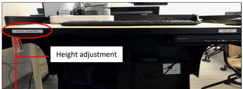
To adjust the height of the console, grasp the adjustment handle and squeeze towards you to release the mechanism. You can then raise or lower the console to desired height.
