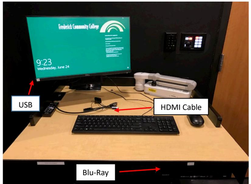
The **Blu-Ray** player is located on the underside of the console top on the right.
