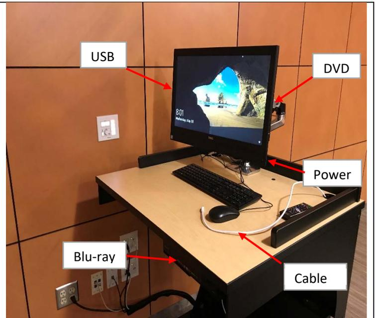
The Blu-Ray player is attached to the underside of the console top on the right.
