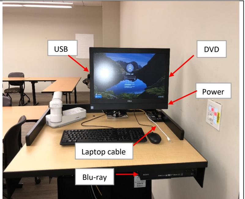
The Blu-Ray player is attached to the underside of the console top on the right.
