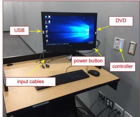
The **USB** ports are located on the left side of the computer screen. If you wish to connect other devices to the projection screen, use the cables on top of the console and press the corresponding button on the A/V controller. Additional **VGA** and **HDMI** cables have been provided.
